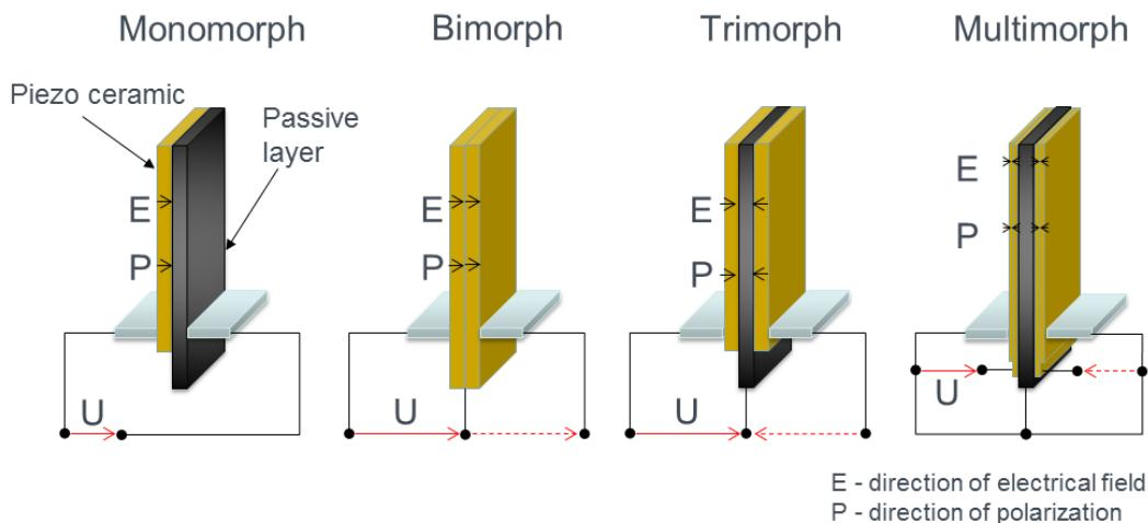
One-sided clamping is normally chosen to make use of the deflection and controlling force at the other end of the bending actuator. The ceramic layers are actuated electrically. The inverse piezoelectric effect gives rise to mechanical stress which results in a bending of the compound.
