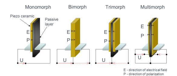
One-sided clamping is normally chosen to make use of the deflection and controlling force at the other end of the bending actuator. The ceramic layers are actuated electrically. The inverse piezoelectric effect gives rise to mechanical stress which results in a bending of the compound.
